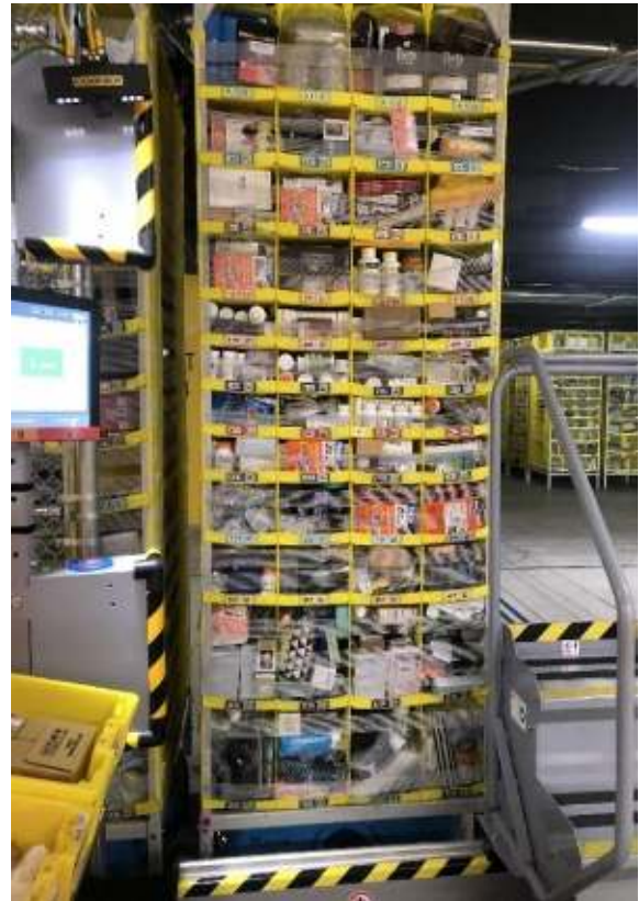
Fig. 6. Pod at workstation for picking. 6
